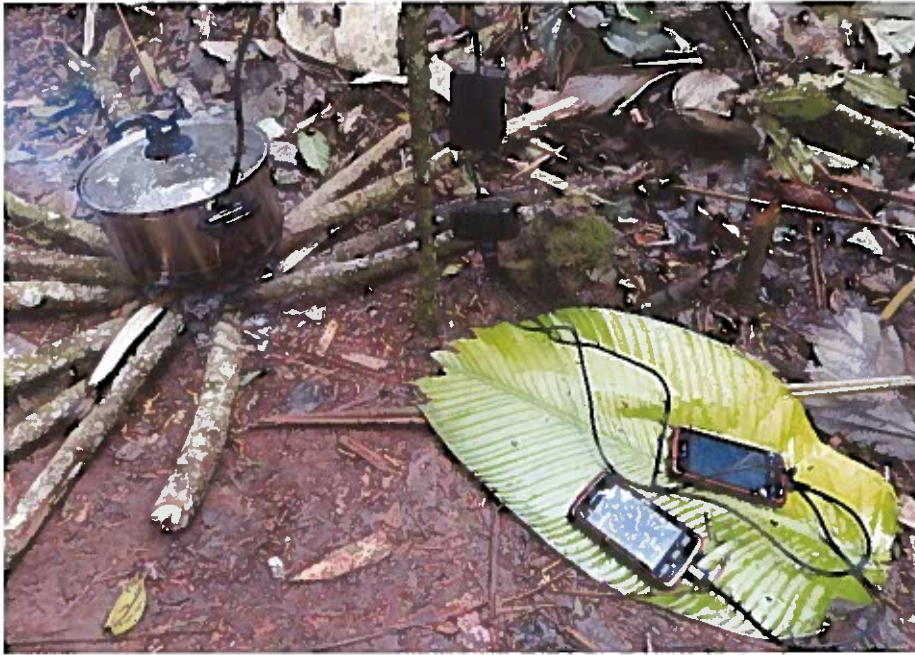
The USB pot charger used to recharge the smartphones (© Julia Altenbuchner)
